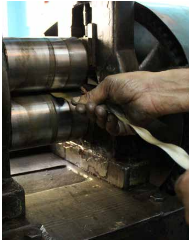
Fig 5.21 Drawing flat silver wire from silver rods in a wire drawing machine
