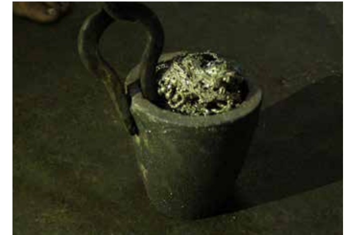
Fig 5.9 Preparing old silver ornaments for melting
