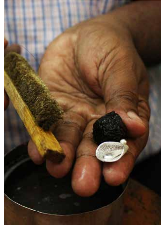
Fig 5.32 Brushing the silver piece using the soap nut
