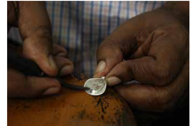
Fig 5.33 Using the curved burnisher to remove the residues
