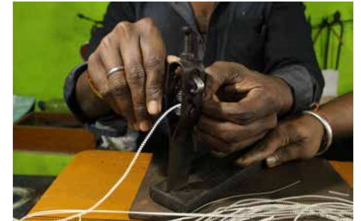
Fig 5.26 Artisan making Janjira with the help of Zig Zag machine.
