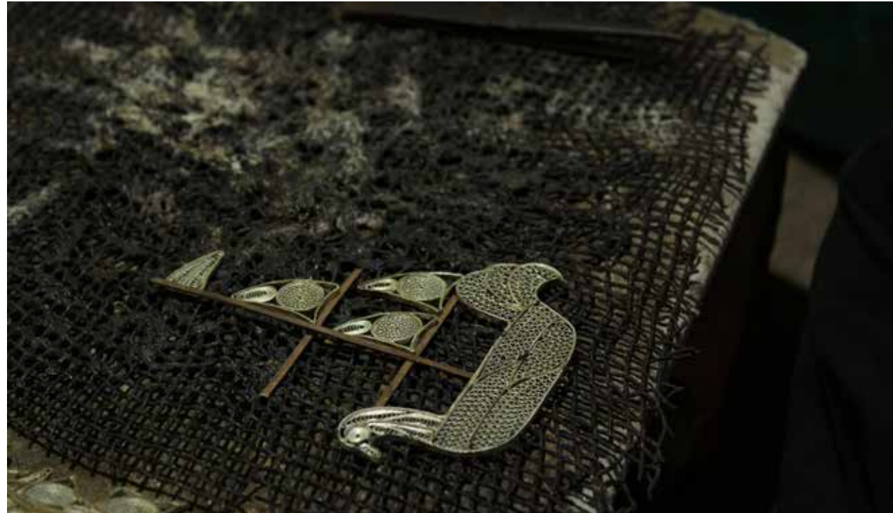
Fig 5.28 Assembling pieces for soldering
