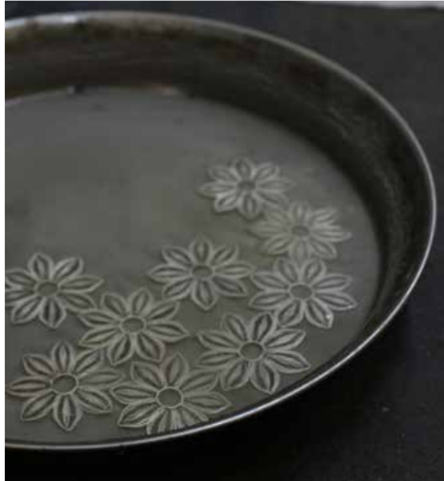
Fig 3.30 Dipping silver pieces in sulphuric acid
