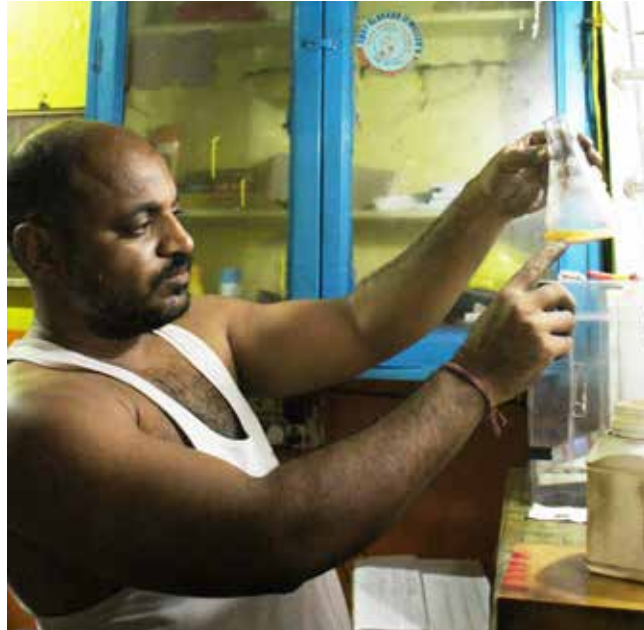
Fig 5.20 Stirring the silver water against titration with Nitric acid
